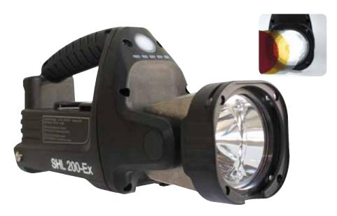
The lamp features a main light, ambient light and flashing light mode, which can easily be activated via the main switch. The main light has a 3W LED which generates a light intensity of 24,000 cd that can also be dimmed.
